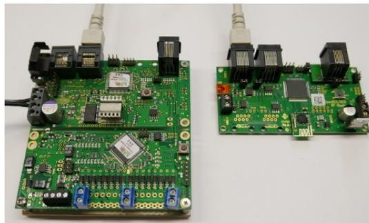
Connected to the BiDiB it is possible to drive, switch functions F0-28 and program decoders CV (POM read and write). For safety reasons, programming of the vehicle decoders by radio is only possible with POM programming commands (targeted to exactly one vehicle). The address CV 1, 17 and 18 can also be programmed in this way.
